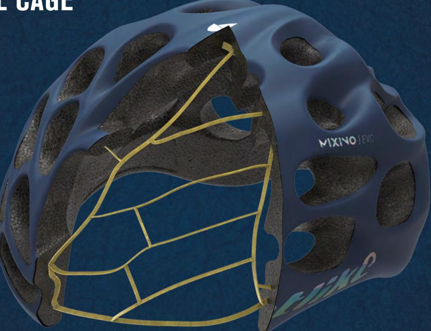
The aramid roll cage is the "skeleton" that works to dissipate the energy of an impact through the whole helmet structure, thus increasing its energy absorption capacity at a reduced helmet volume and weight. This structure will also help to hold the helmet together in the event of a crash.
